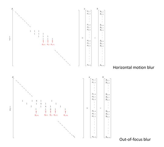
The task of this project is to recover sharp image X from the blurred version B, given the blurring operator A.
